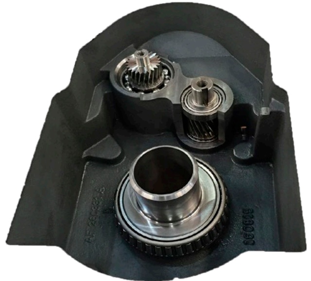
COMPACT SERIES INTERNALS Triple Reduction and Dry Well
